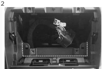
2 Cut and remove the plastic parts along the dotted white line in the figure.
