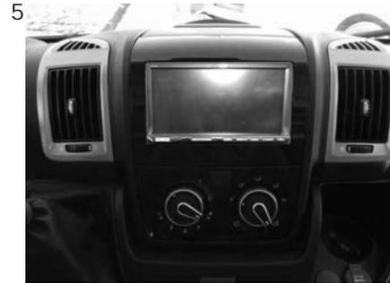
5 Connect all cables, verify the proper functioning of the system and insert the radio-frame into the housing.
