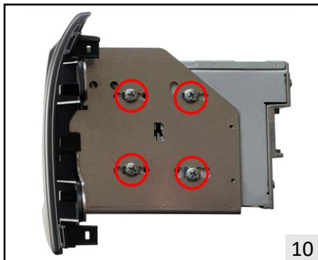
10. Fix the fascia plate to the radio by tightening the 8 screws (4 per side) supplied in the kit.
