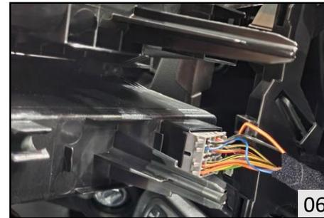
6. Disengage the ISO connector from the OEM radio dock.
