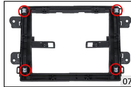
7. Remove and save the 4 clips circled found to the back side of the OEM fascia plate.
