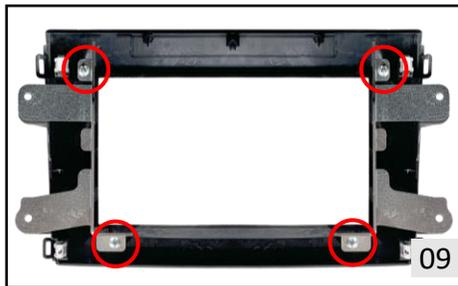
9. Fix the metal brackets to the fascia plate by tightening the 4 screws (2 per side) supplied in the kit.
