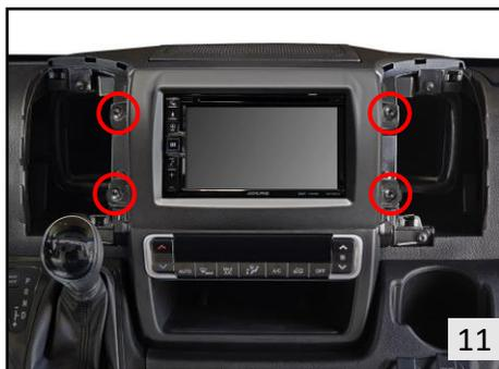
11. Make all connections. Check the proper functioning of the whole system. Fix the head unit with the OEM screws saved in the step n°4 as indicated in the picture.
