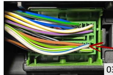
03 The White/Blue cable (Pin 17) carries the reverse signal in the Green connector. Remove the terminal from the connector housing.
