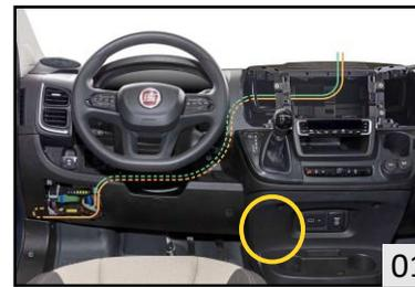
01 Routing of the speed & reverse cable and a position of Grey connector (3)
