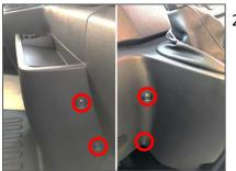
2. Unscrew and save the 4 screws circled in Red and remove the plastic panel.
