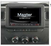
Install the panels you have removed and install the fascia plate supplied in the kit.
