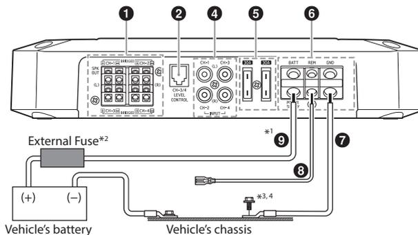
\*1 For details on the wires size to be used, refer to the supplied "Cautions on Power Supply Wires Connection" and "Cautions on Power Supply Wires" (page 20), and then use the wire of the specified size.
