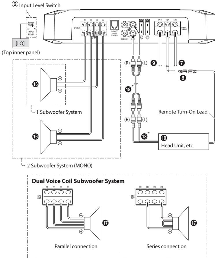
\* If the connected head unit does not have an RCA Output and RCA Extension Cable (18) cannot be used, you can use the Speaker-RCA Conversion Cable (19) (sold separately). For details on how to make a connection, see "About Connecting to the Speaker Input Level System" (page 19).
