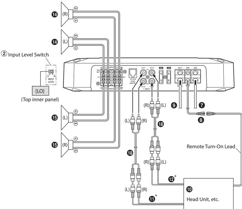
\* If the connected head unit does not have an RCA Output and RCA Extension Cable (18) cannot be used, you can use the Speaker-RCA Conversion Cable (19) (sold separately). For details on how to make a connection, see "About Connecting to the Speaker Input Level System" (page 19).
