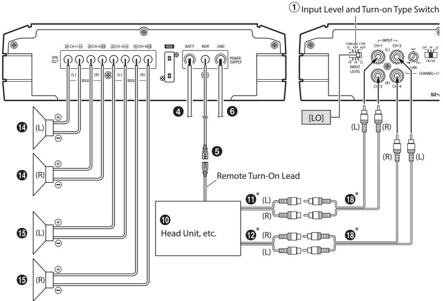
\* If the connected head unit does not have a Speaker Output and RCA Extension Cable (18) cannot be used, you can use the Speaker-RCA Conversion Cable (19) (sold separately). For details on how to make a connection, see "About Connecting to the Speaker Input Level System" (page 16).
