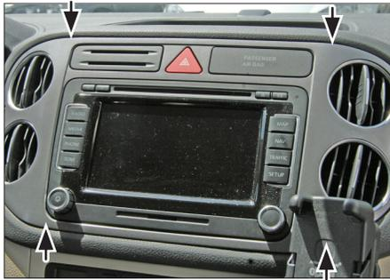
1. Unclip and remove OEM panel (see arrows)
