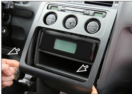
1. Unclip and remove OEM panel
