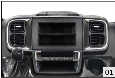
1. This is how the original dashboard looks like once removed the radio panel.
