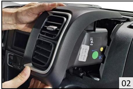
2. Disengage both air vents with a removal tool and remove both air vents.
