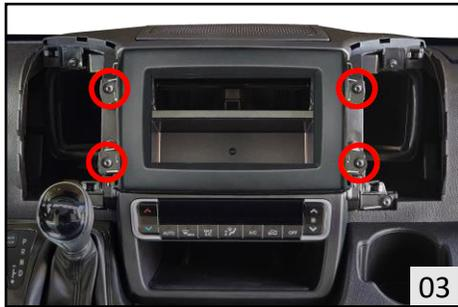
3. Remove and save the 4 screws circled in Red. Disengage the ISO connector from the OEM fascia plate.
