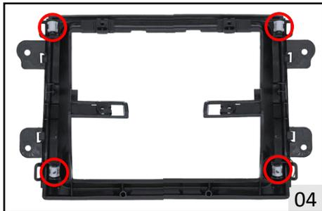
4. Remove and save the 4 clips circled found to the back side of the OEM fascia plate.
