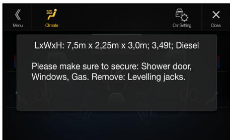
*The Pre-Flight Check features shows the vehicle parameters and preselected warnings every time the engine is started.*
