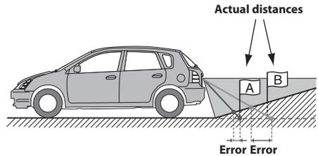
The distance guidance mark represents the distance to a flat road surface. Therefore in the case of an upward slope the distance guides are displayed closer to the rear bumper than the actual distance. For example, if there is an obstacle on the upward slope, it may appear farther away than its actual position.
