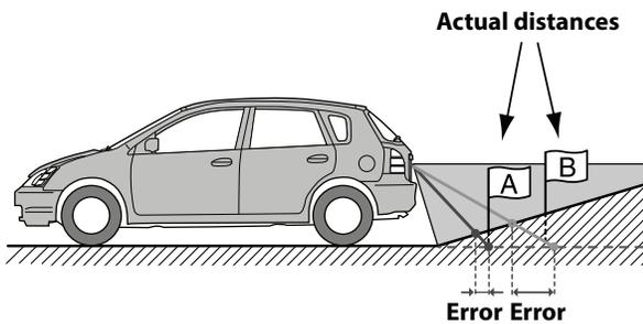
The distance guidance mark represents the distance to a flat road surface. Therefore in the case of an upward slope behind the car, the distance guides are displayed closer to the rear bumper than the actual distance. For example, if there is an obstacle on the upward slope, it may appear farther away than its actual position.
