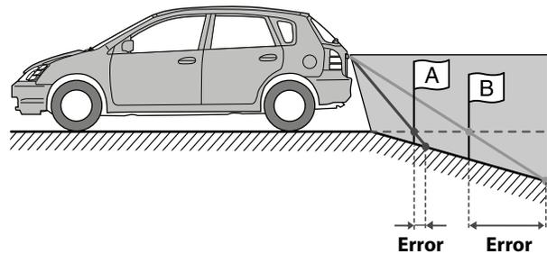
In the case of a downward slope behind the car, the distance guides are displayed farther from the rear bumper than the actual distance.
