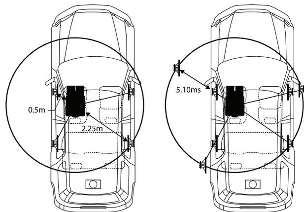
The sound is not balanced because the distance between the listening position and the various speakers is different. The difference in distance between the front left speaker and the rear right speaker is 1.75 m (68-7/8").
