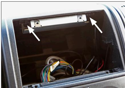
4. Assemble speed nuts on mounting plate
