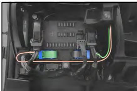
Position of fuse box and the two terminals for speed and reverse connection.
