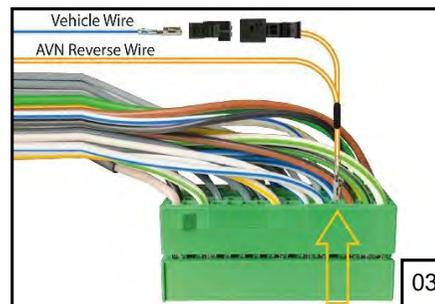
03 Use the supplied Y-cable of the main cable harness.
