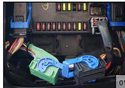
01 Disconnect the two lower 60-pin connectors.
