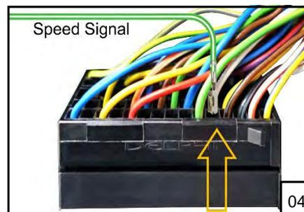
04 Remove the black connector cover on the same principle as the green connector and plug the speed signal cable into the free chamber 56.
