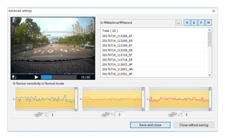
Advanced sensitivity settings allows you to fine-tune the event recording G-Sensor threshold, while watching pre-recorded G-Sensor data and video as a reference.
