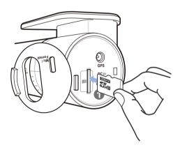
Peel off the plastic film from the dashcam. Peel off the protective film from the double-sided tape and attach the dashcam to the windshield behind the rear-view mirror.
