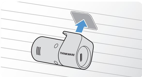
Attach the product with the THINKWARE logo facing indoors and press the adhesive tape firmly to secure the camera.
