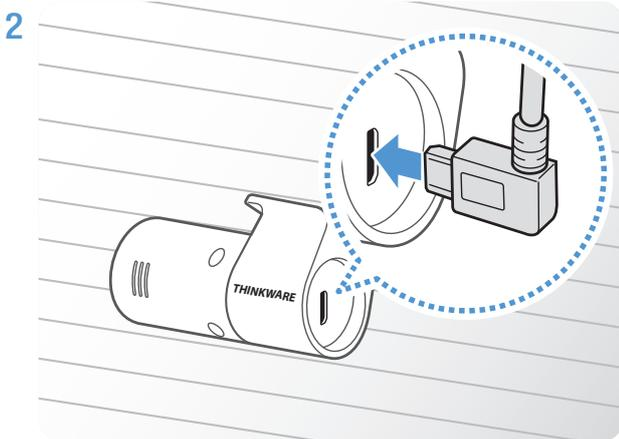
Connect the other end of the rear camera cable to the rear camera's connection port.
