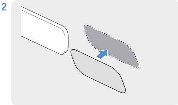
Attach the heat blocking film to the installation location.
