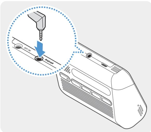
Connect the RADAR module to the product's RADAR connector.
