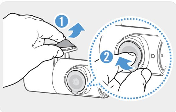
Remove the protective film from the adhesive mount and camera lens.
