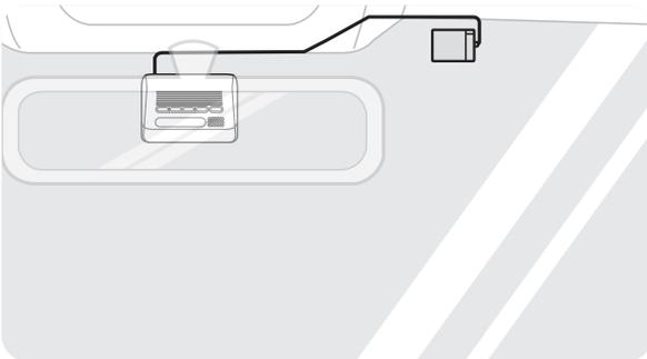
Attach the RADAR module's adhesive surface to the upper part of the front windshield and press the adhesive part firmly to secure it.
