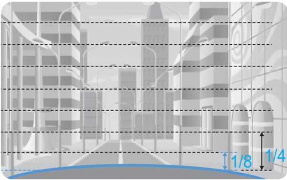
Connect the product to **THINKWARE DASH CAM LINK** on your smartphone and adjust the camera angle so that the hood of the vehicle covers  $1/4 - 1/8$  of the screen while viewing the live view screen, as shown in the image to the left.
