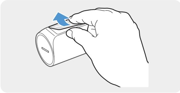
Remove the film on the back of the RADAR module.
