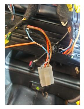
The purple wire for the reverse feed is for switching to an aftermarket reverse camera if fitted when the vehicle is put into reverse gear.
