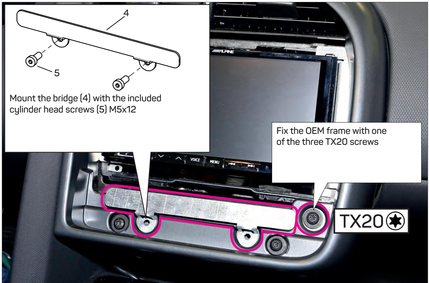
Mount the bridge (4) with the included cylinder head screws (5) M5x12
