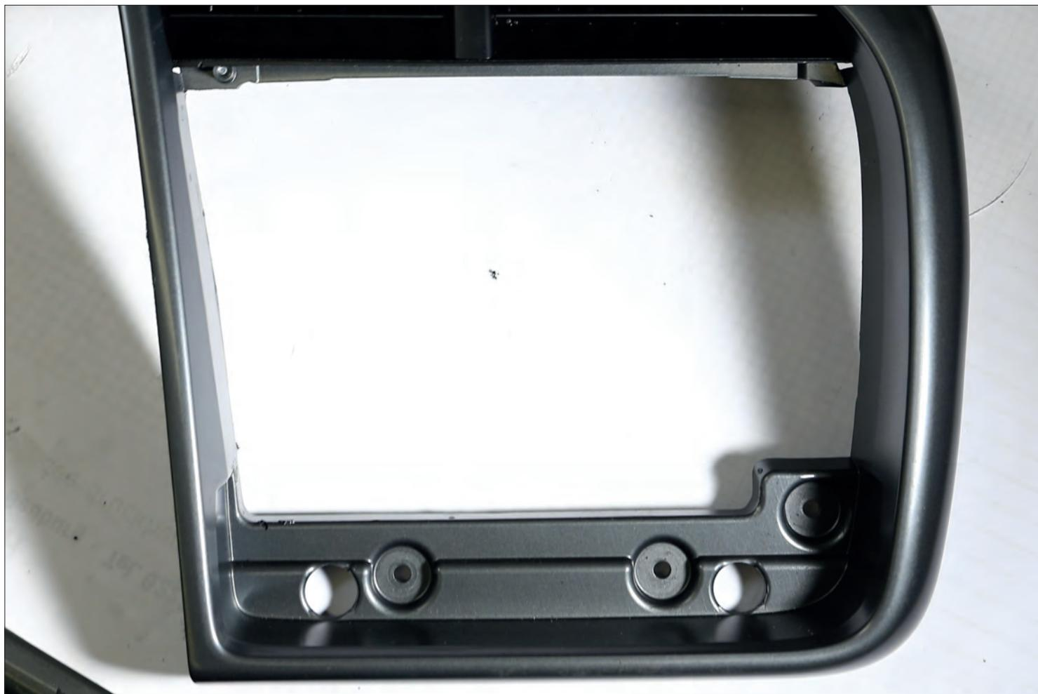
Attach the mounting frames with the included flat headed screws to the 2-DIN headunit. We recommend a distance of app. 16 mm to the front of the head unit
