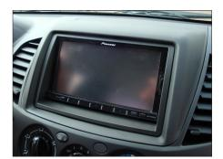
7. Place OEM-Panel onto dashboard to finish installation
