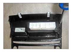
Remove hazard light switch and display from OEM bezel
