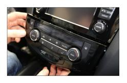
I. Unclip air condition control unit under OEM head unit
