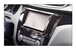
10. Put clips on the rear side of facia plate. Place facia plate on dash board
