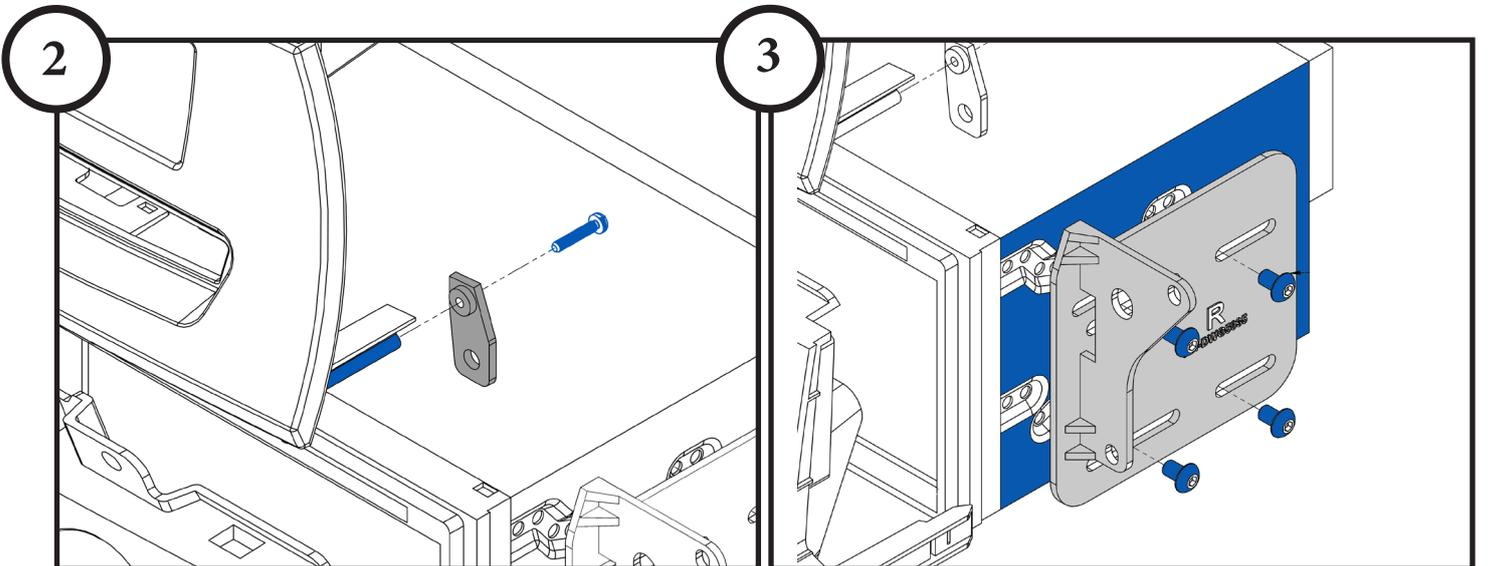
Screw each relocation mount into place at the bottom right and left corners of the upper panel using the x2 Pozi Pan screws included with the kit
