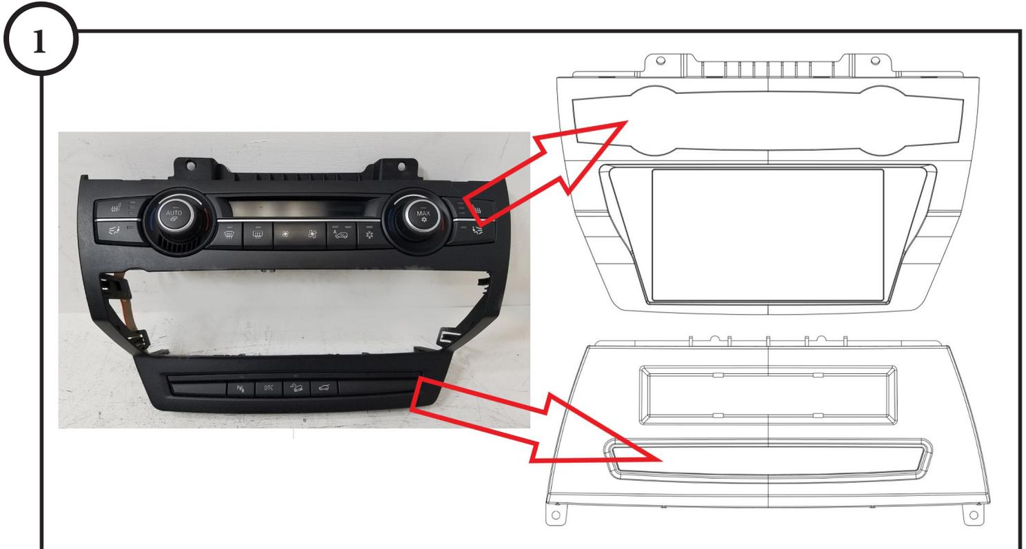
Relocate the climate control panel and switch panel from the OEM piece (left) to the top and bottom aftermarket pieces (right) as shown in the image. Remove the clips from the OEM piece and relocate them to the aftermarket fascia panel.
