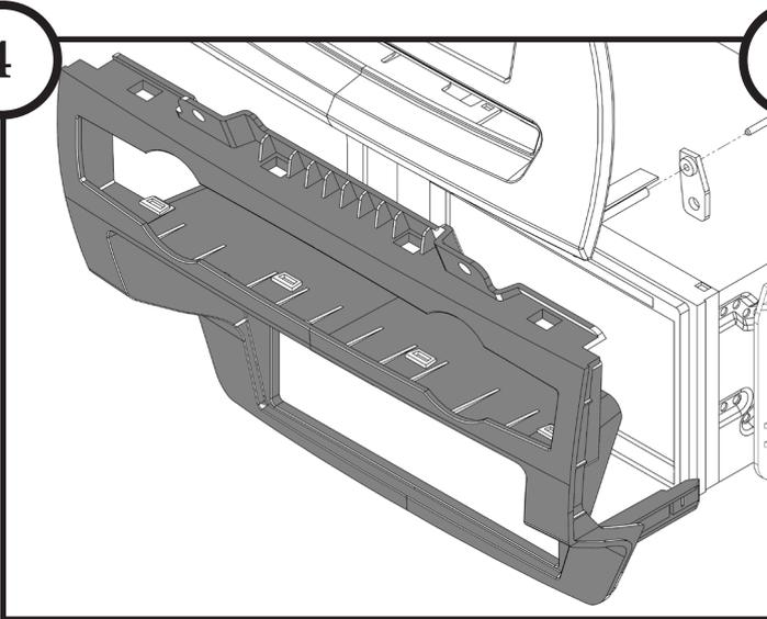
Surround the head unit with the lower panel and lock into place using the clips retained from the OEM panel and the OEM screws.
