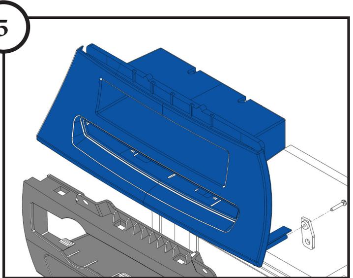
Place the upper panel into the dashboard and secure in place using the OEM screws.
