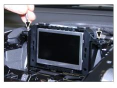
Remove two TX20 screws of display Remove display
