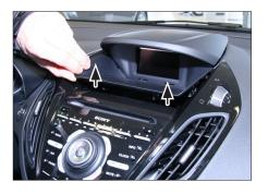
Unclip and remove panel on top of B-MAX dashboard (see arrows)
