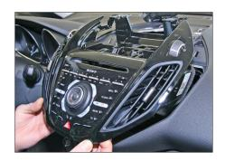
Unclip and remove center console
