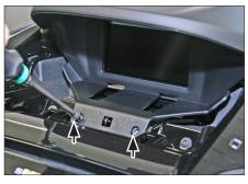
Remove screws of display panel (see arrows) Remove display cover
