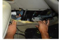
pin switches 1-4 according to the brand of new head-unit you are fitting. The extra cables on this interface are for ignition output, illumination, speed pulse and park brake if needed.
