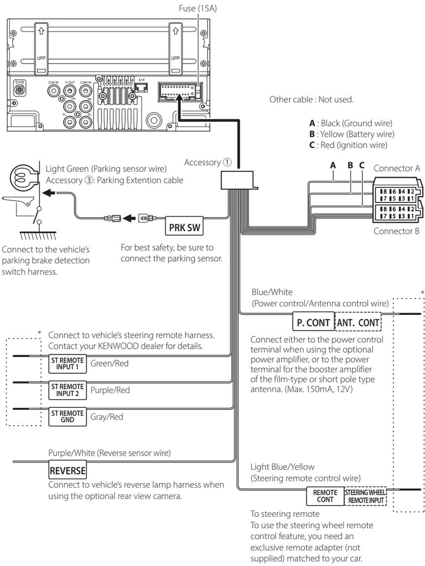
\* Do not remove the cable from the heat shrink tubing unless you are making a connection.
