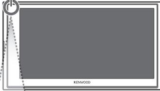
\* DO NOT expose the remote sensor to bright light (direct sunlight or artificial lighting).
