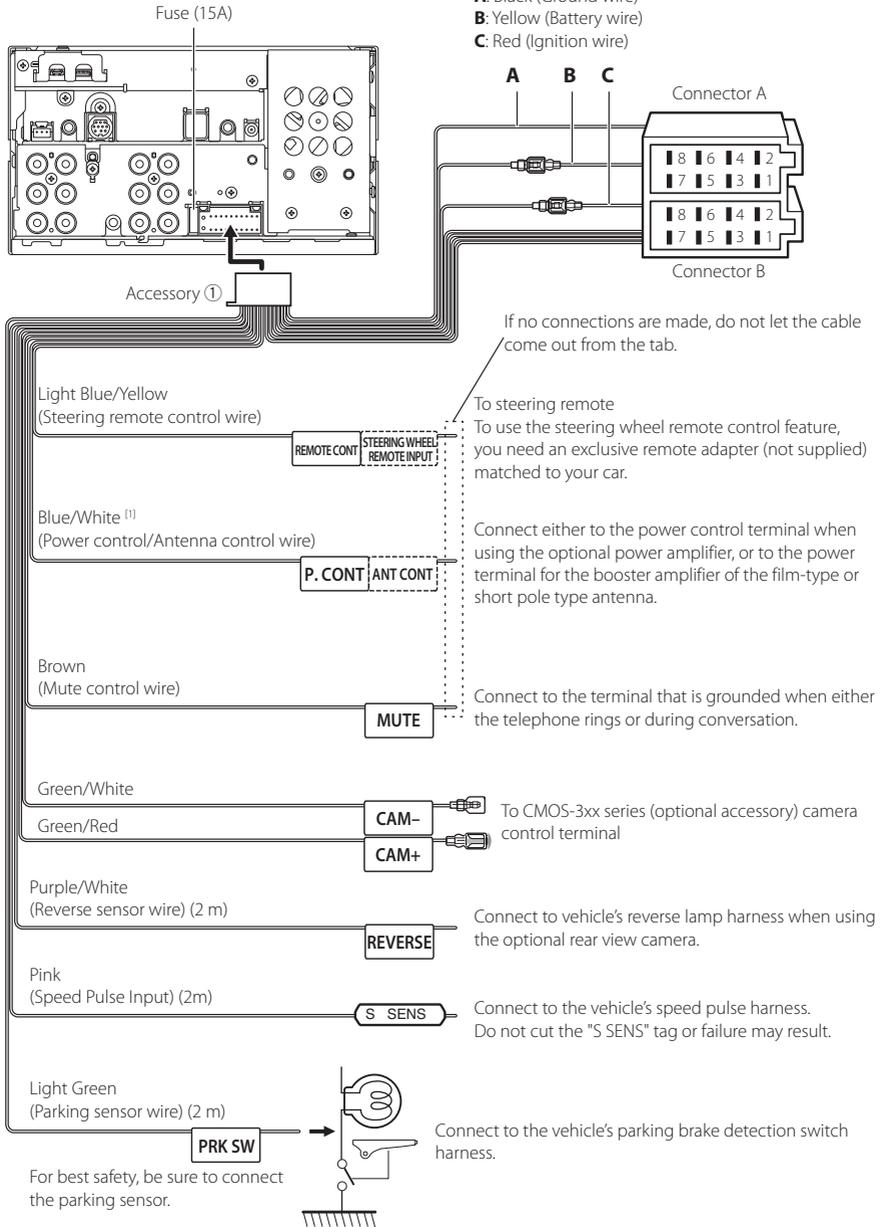
[1] [2]: Blue/White wire is provided two wires, [1] and [2]. Blue/White wire total output ([1] + [2]): 12 V  $\approx$  350 mA
