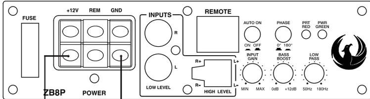
**NOTE:** In this connection, the **AUTO POWER ON** switch is in the **ON** position.
