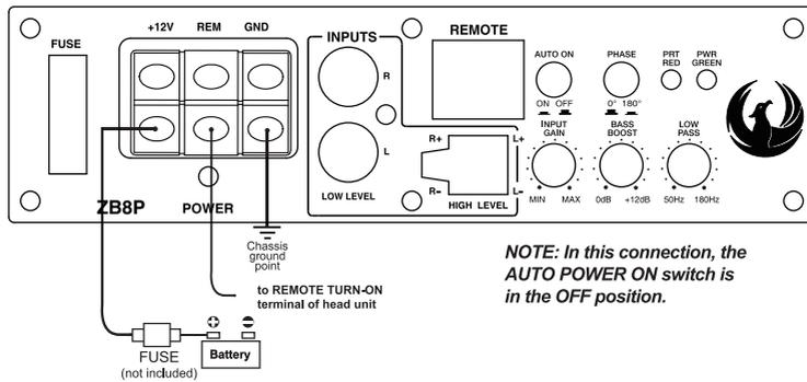
**NOTE:** In this connection, the **AUTO POWER ON** switch is in the **OFF** position.
