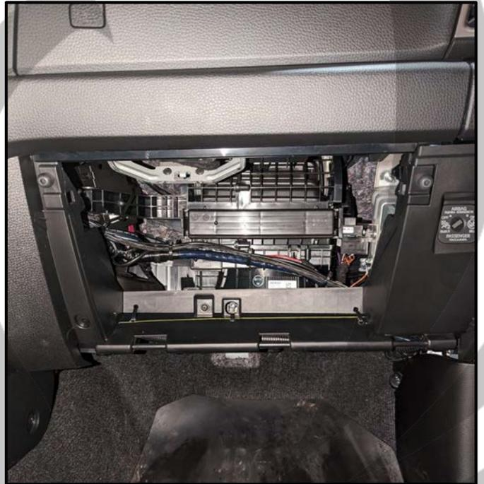
15. Remove the threshold panel
