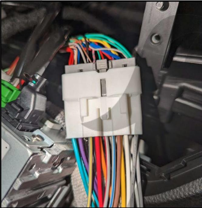
10. Connect SOT cable to stereo
