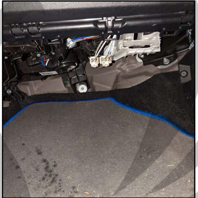
19. Remove the threshold panel
