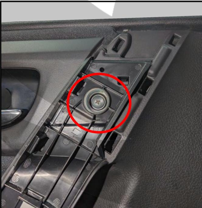
8. Remove the window switch panel
