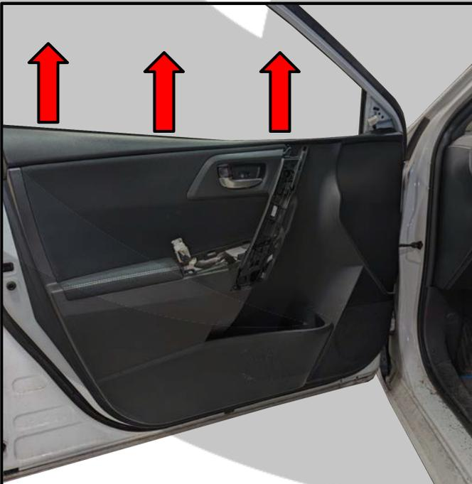
12. Remove the door opener cables
