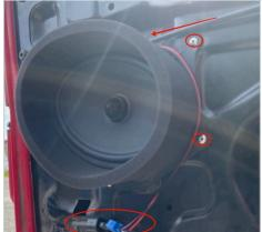
Place the speaker with the new frame in the original place and position the new speaker cable on the top side of the frame.
