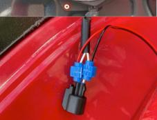
The plug on the top of the harness is positive and the lower plug is negative.
