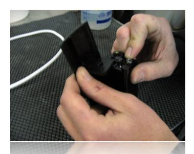
Make sure to keep an eye on the spring as you unclip the door, as it can uncompress quickly and will be hard to find if it pops off. Also carefully note its orientation, as you will need to remember this for reinstallation onto the spec.dock.
