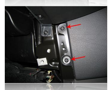
Removing the side panel reveals two Torx T-20 screws. Remove these.
