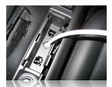
Run the wiring from the spec.dock through this hole as shown.
