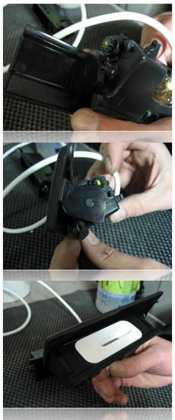
Continue by reinstalling the spring in its original orientation and snappng the door completely onto the spec.dock as shown.
