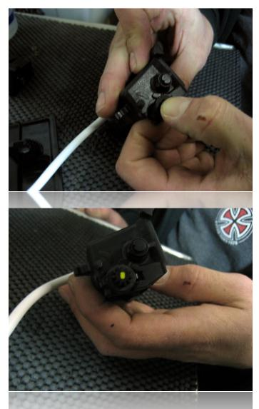
Snap the geared roller into the same position on the spec.dock.
