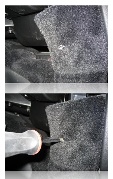
Begin by removing the single Torx T-27 screw buried in the carpeted panel on the side of the center stack.
