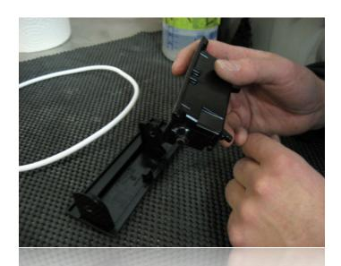
The door is now free from the ashtray base. You should keep the OEM piece as it may be needed to reverse the spec.dock installation later if ownership of the car is transferred.
