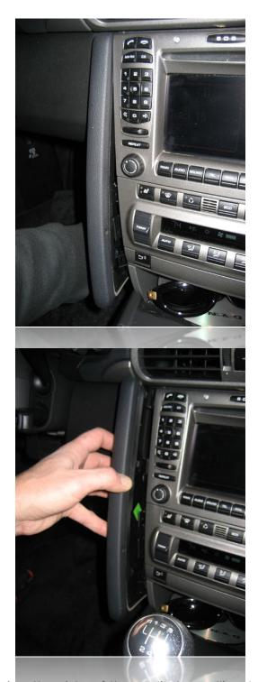
Remove the panel covering the side of the radio by pulling toward you and out. It will snap completely free of the vehicle. Set aside.
