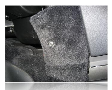
Once this screw is removed, this panel simply snaps out. Set aside.
