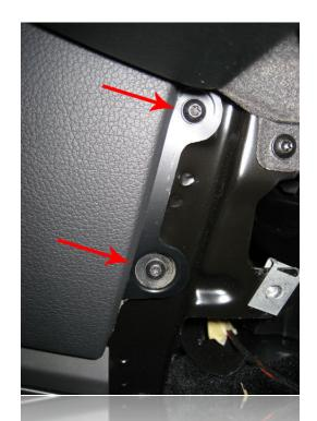
Again this will reveal two Torx T-20 screws that need to be removed.
