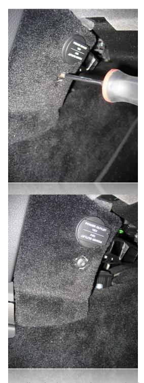
Similar to the left side, remove the single Torx T-27 screw buried in the carpeted panel on the right side of the center stack.
