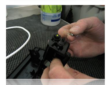
Carefully remove the spring from the OEM ashtray base and set aside.
