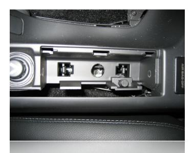
Drill a small hole (roughly 3/4") into the ashtray housing in the location shown for routing of the spec.dock's wiring. Make sure to check for any harnesses that may be located under this spot before drilling and move them out of the way.
