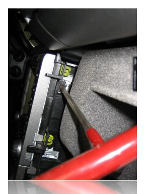
On the right side of the radio, you will see two Allen-head screws. These need to be turned 1/4 rotation to depress the locking tabs that hold the radio in place.
