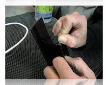
Start by gently prying up on the side of the ashtray lid with the spring and geared roller using only your fingers. The plastic lid will give a little and slide off of the hinge pin.
