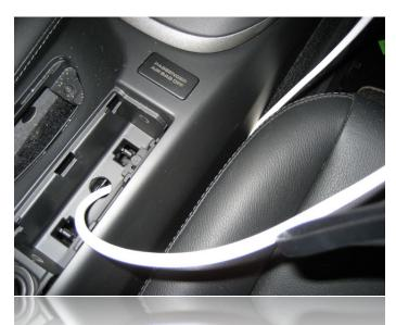
You should be able to reach under the right side of the center console to grab the wiring from the spec.dock. Pull it through as shown, and continue pulling the slack on the cable as the spec.dock is lowered into position and snapped into the ashtray location.
