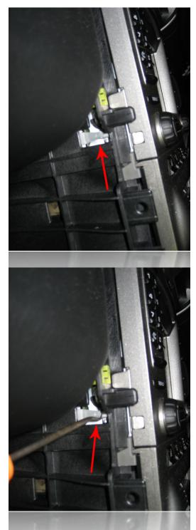
The locking tabs on the left side of the radio are a bit more difficult to access without removing the driver's side knee panel, but possible. These can be depressed with a dental pick tool while gently pulling out on the radio face. There is also one clip above the one pictured here.
