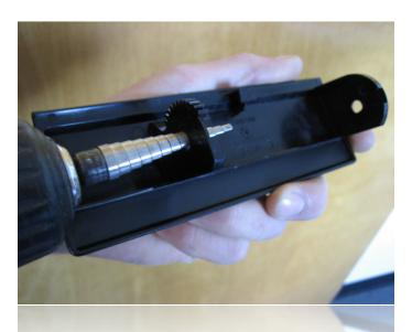
This step is only required in SOME Type 997 applications. If your ashtray door already has large holes for the hinge pins, you will not need to perform this step. If the holes for the hinge pins are small, carefully open them up using a UniBit step-drill to 1/4" diameter. A regular drill bit is not recommended, as the holes may get off center if they are not carefully enlarged. The UniBit is best for this.
