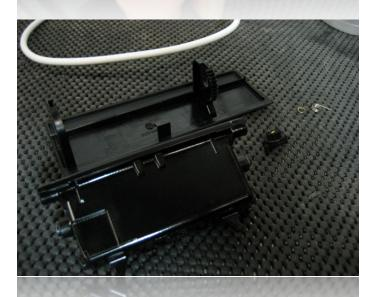
This is what you should end up with before assembly of the spec.dock - OEM ashtray base, door, geared roller and spring.
