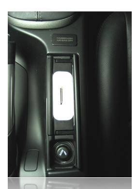
The properly installed spec.dock should look like this. Make sure to test the functionality of the door mechanism and the interface before completely reassembling the vehicle. Reassembly is the reverse of disassembly.
