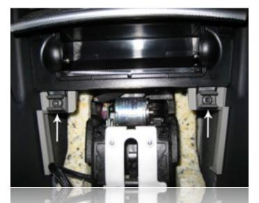
Remove the two torx T-20 screws indicated here. This will allow the ashtray carrier to be lifted up and out of the console.
