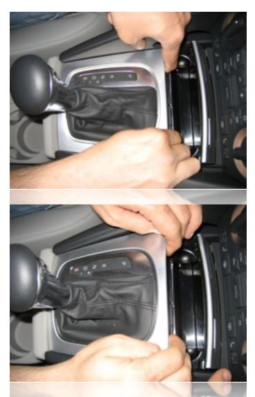
Begin by using your fingers to unsnap the trim around the shifter by pulling up on the front lip of this piece as shown.
