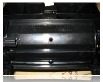
Place the ashtray carrier face-down on a soft surface and drill a small pilot hole in the location shown.
