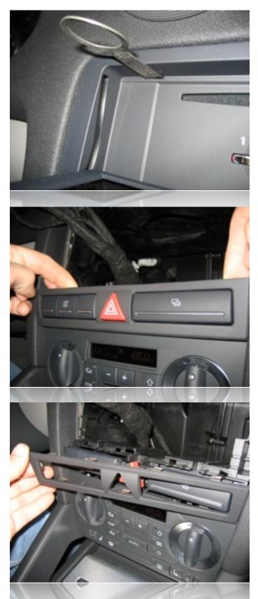
Using only your fingers, gently unsnap the trim around the hazard switch and storage pocket. Remove this piece completely and set aside.
