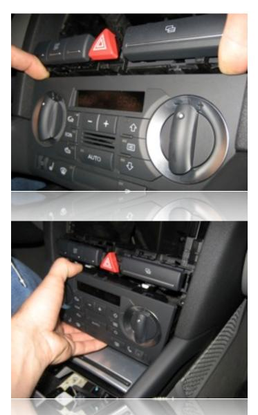
Again using only your fingers, snap the climate control panel out of the dash as shown. It is not necessary to disconnect the connectors on the back of the climate control, as the wiring length allows it to easily move out of the way. Once this unit is removed, the radio can temporarily be slid back into the dash.
