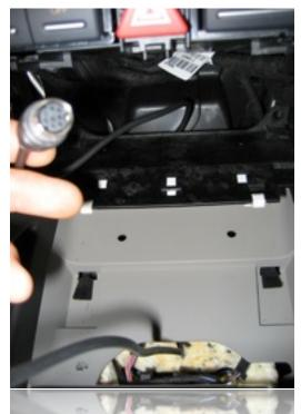
When reinstalling the ashtray carrier with the spec.dock mounted back into the vehicle, route the cabling as shown above. This will make it very easy once the ashtray carrier is back in place to run the wiring up to the radio location where the interface electronics will be located.
