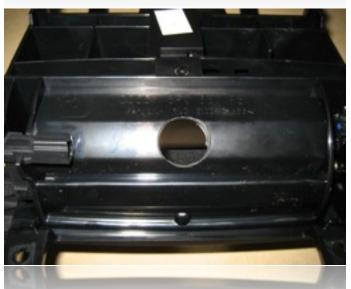
This hole will need to be opened up to 3/4" to allow the spec.dock's wiring to pass through.
