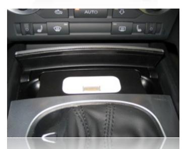
Your spec.dock is now installed and can be connected to the interface electronics according to the instructions included. Make sure to test all functionality before completely reassembling the vehicle. Reassembly is the reverse of disassembly.
