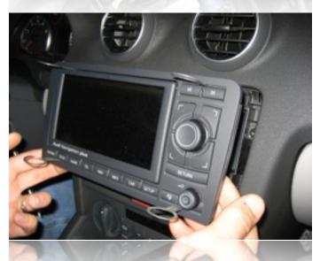
Using Audi radio removal keys, slide the radio out of the dash as shown. If the car is equipped with a navigation unit, note that the fourth key slides in behind the screen.
