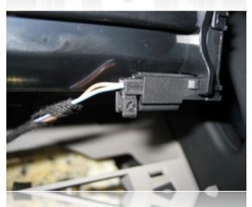
Make sure to disconnect the connector on the bottom side of the ashtray carrier so that it can be removed completely from the vehicle.
