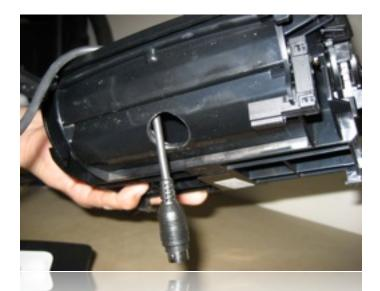
Route the wiring from the spec.dock through the hole you just cut.
