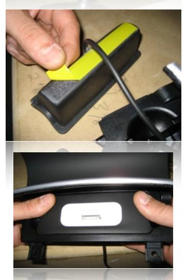
Remove the backing from the included double-sided tape and lower the spec.dock into position, pressing down firmly as shown.
