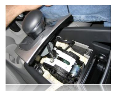
Completely remove the shifter trim and set aside.
