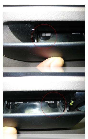
Your first step will be to remove the factory ashtray insert and to locate the two spring clips located in the spots indicated in the above photos.
