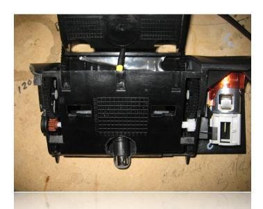
Thoroughly clean the inside of the ashtray housing with a high-quality degreaser such as denatured alcohol, and then route the integrated cable from the spec.dock through the hole you just created. You can then remove the backing from the double-sided tape on the back of the spec.dock and press it firmly into place. You are now ready to reinstall the ashtray housing with the installed spec.dock back into the car.
