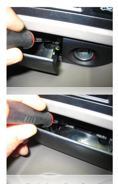
Use a small flathead screwdriver to depress these clips as shown while gently pulling toward you on the ashtray drawer itself to unclip the assembly from the dash. It is usually best to unclip one side at a time.
