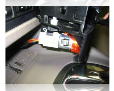
There is one electrical connection to this piece at the cigarette lighter. Unplug this connector and remove the ashtray assembly from the vehicle.
