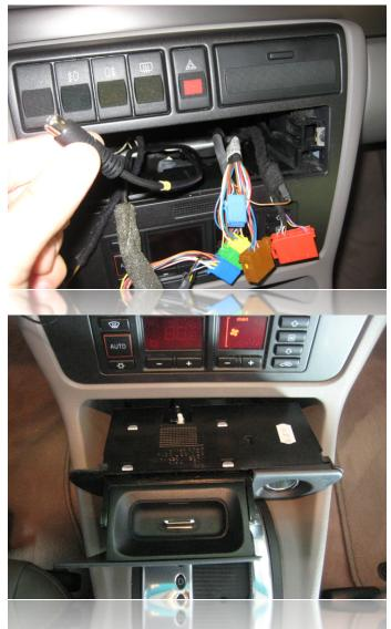
Pull the spec.dock cable up through the radio opening, and pull the cable slack into the radio opening as you slide the ashtray housing into place. Make sure not to pull the cable too taut, as there needs to be a small amount of slack to allow the ashtray drawer to slide in and out.
