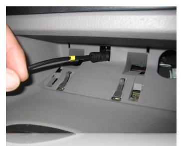
Route the spec.dock cable through the hole in the vehicle console shown above. This is very important, as it will ensure proper operation of the ashtray drawer.
