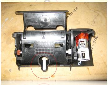
Using a hole saw or Unibit, cut a 3/4" hole in the exact location shown, taking car not to damage the ashtray drawer locking mechanism, which is the white lever seen in this photo.
