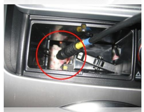
Remove the original ashtray insert and run the spec.dock's integrated cable through the existing opening in the ashtray well as shown.
