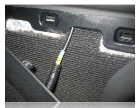
You will easily be able to grab the end of the cable through this opening on the side of the console where you removed the panel earlier.
