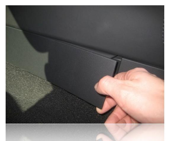
Begin the installation process by using your fingers to unsnap this panel on the side of the center console.
