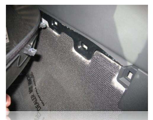
This panel will continue to unsnap toward the front of the vehicle. You won't need to remove it completely - just releasing these three clips will give you all the room you need to route the spec.dock cable.
