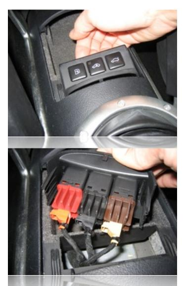
With the switch panel removed, unplug the three connectors on the backside of the panel and set aside.
