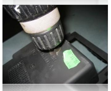
Enlarge this hole to 1/2" using a Unibit step drill bit or a hole saw.
