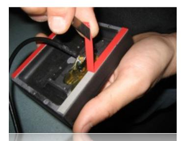
Remove the backing from the pre-installed double-sided tape on the spec.dock.
