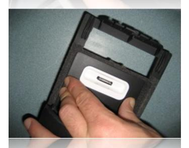
Lower the spec.dock into position while pulling through any remaining slack on the integrated cable and press down firmly to ensure proper adhesion. You will now be able to connect the spec.dock cable to your interface electronics and test all functionality before reassembling the vehicle interior. Reassembly is the reverse of disassembly.
