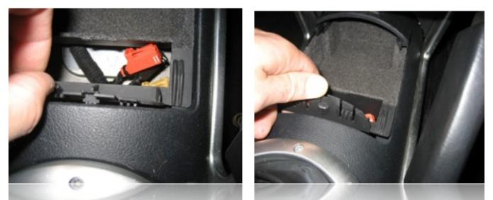
Next, use your fingers to start unsnapping the clips on the front edge of the storage pocket that hold this piece in place, which were revealed when the switch panel was removed.
