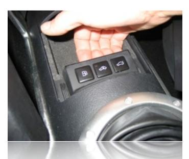
Begin by reaching behind the switch panel in front of the shifter and lifting up gently using only you hand. This panel will easily begin to snap out of its location.
