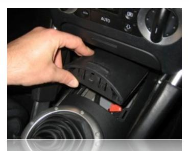
This will allow you to completely remove the storage pocket by lifting up and toward you. Make sure the door on the storage pocket is closed so that the entire unit will clear the surrounding dash trim.
