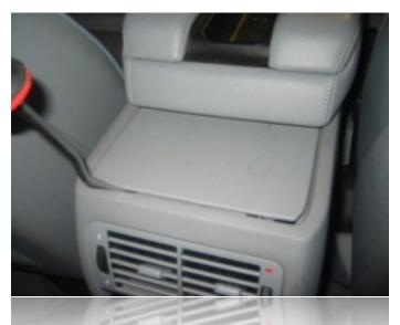
Begin by using a panel tool to pry up the leather-wrapped panel located at the back of the center console underneath the sliding armrest. The armrest will need to be slid forward completely to remove this panel. The clips that hold this panel in place are very brittle, so be as gentle as possible. Set this panel aside.
