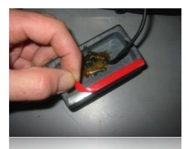
Remove the backing from the included double-sided tape on the bottom of the spec.dock. Before dropping the spec.dock into place, make sure to clean the ashtray carrier thoroughly with a high-quality degreaser such as denatured alcohol. This will promote proper adhesion of the tape. Make sure to press down firmly on the spec.dock for a few seconds once it is in position.
