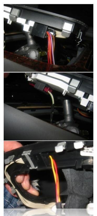
There are three plugs connected to the shifter trim that need to be unplugged so that the piece can be completely removed. Once these are disconnected, fully remove the shifter trim and set aside.
