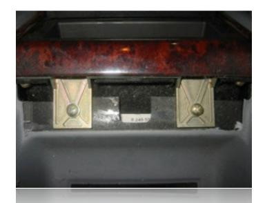
Removing the armrest reveals two brass screws that hold the top of the center-console woodgrain trim in place. Remove these.
