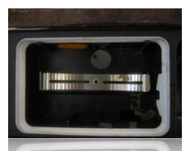
This is what the hole you just drilled should look like from the top. Make sure to clean any plastic debris out of the ashtray carrier before repeatedly opening and closing the door to avoid any problems with the mechanism.
