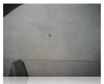
Returning to the vehicle, you will want to remove the single Philips-head screw located in the left side of the center console next to the gas pedal.
