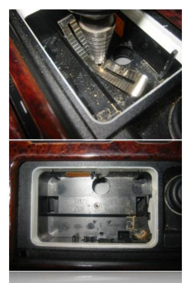
Before the spec.dock is installed, the factory ashtray spring will need to be removed as well. This is accomplished by drilling the head out of the rivet that holds this spring in place. Once the head is drilled out, the spring will be easily removed.
