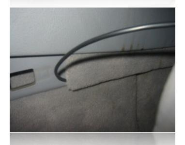
Route the wiring from the spec.dock through this spot in the side of the center console and connect to your interface electronics according to the instructions included. Make sure to test all functionality before completely reassembling the vehicle.
