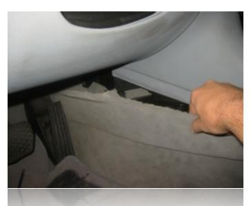
Now, using only your hands, pull the front of this panel out slightly while sliding it toward the front of the car to release the clips that hold the console side panel trim in place.
