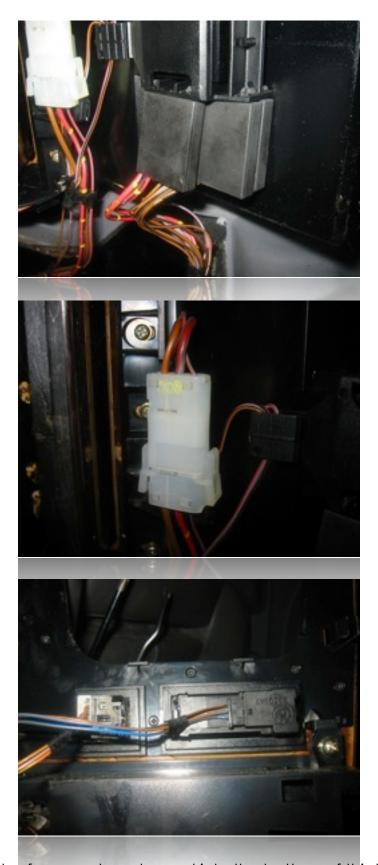
There are three sets of connectors plugged into the bottom of this trim piece. Unplug all of these so that the piece can be completely removed from the vehicle.
