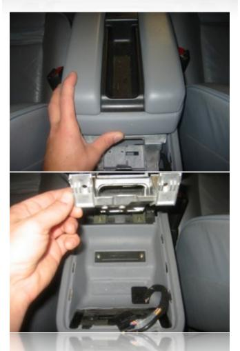
Push forward on the armrest to slide it out of the retainer. You will be able to easily lift it up and away from the console. Set aside.
