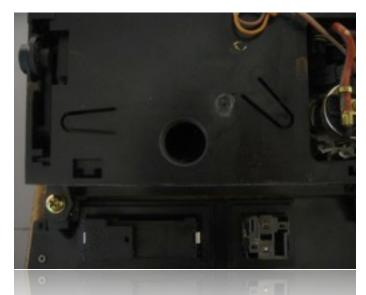
Place the center console trim upside-down on a well-lit work surface. **Make sure that the ashtray door is closed before proceeding**. You will be drilling a 1/2" hole in the
