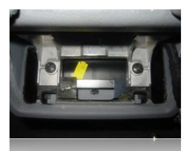
You will see two large Philips-head screws that are revealed with this panel out of the way. Remove these and set aside.
