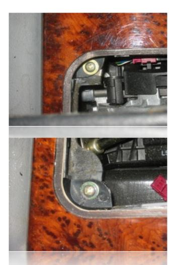
Under the shifter trim, you will find two more brass Philips-head screws that need to be removed.
