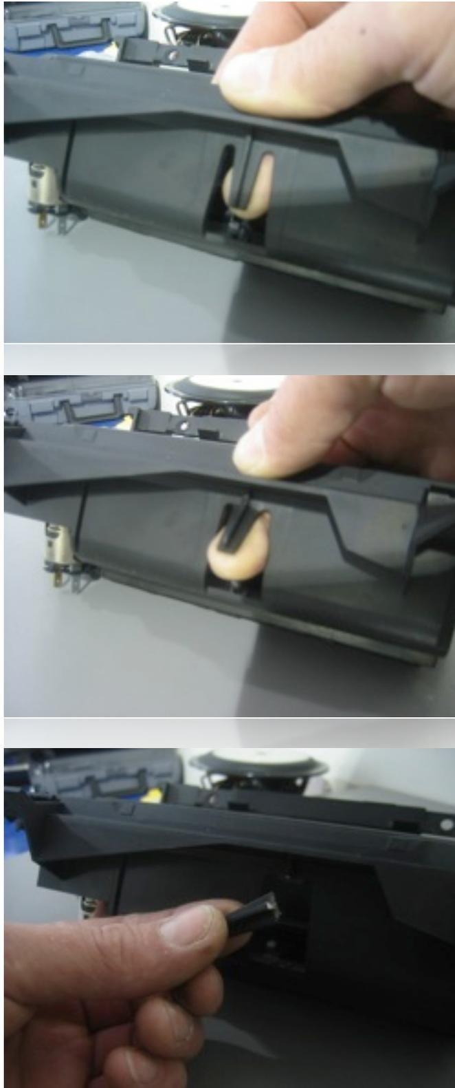
The wiring from the spec.dock will exit through this factory opening. Using your finger, push the tab outward to snap it off. This tab performs no locking or cosmetic function, so the factory ashtray can still be reinstalled at a later date.
