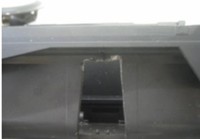
Depending on which interface cable is installed, it may be necessary to cut a small amount of plastic out of the way to allow the spec.dock to drop into the ashtray well.
