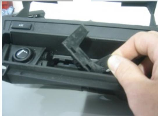
The ashtray lift needs to be removed to keep it from trying to pop the spec.dock out of position, and to allow the ashtray door to open more to accommodate the iPod when docked. Using only your fingers, gently pull this piece toward you. It unclips from the ashtray carrier itself.
