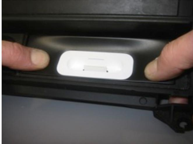
Once the spec.dock is in position, press down firmly on either side of the dock to ensure full adhesion.
