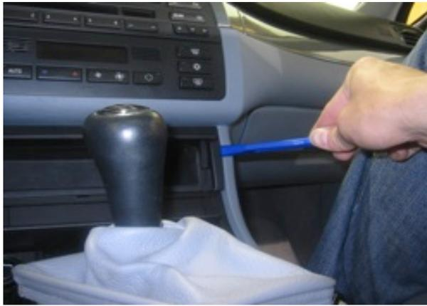
Next, use a plastic dash trim tool to release the clips on the storage pocket below the climate controls. Make sure not to use too much pressure, as the dashboard itself can be damaged if great care is not used. Usually, once one side is freed, the pocket can simply be slid out.
