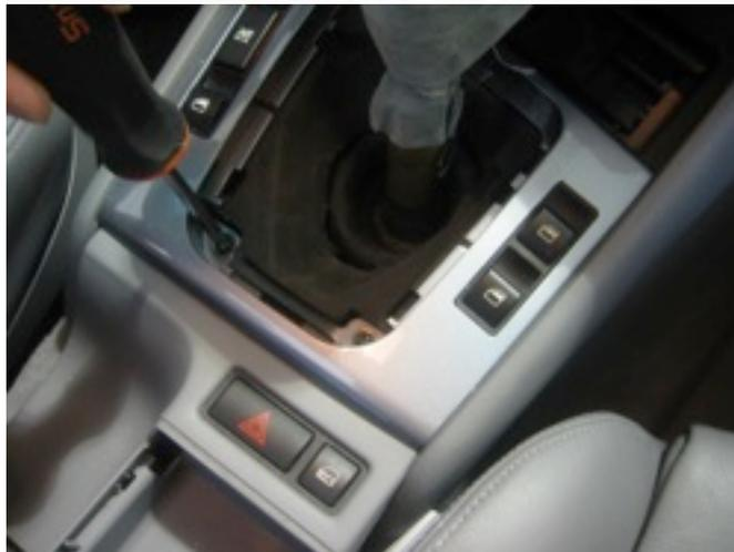
Underneath the shift boot and its former are two Philips-head screws. Remove these to allow removal of the shifter trim.
