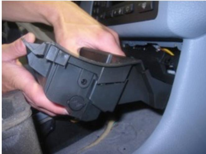
The ashtray carrier can now be removed by pulling toward the back of the vehicle while lifting up on the back of the piece to clear the shifter.
