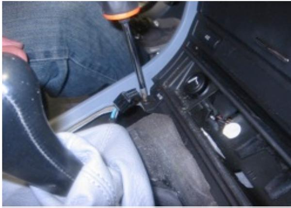
Under the shifter trim are two more Philips-head screws that need to be removed to allow the ashtray carrier to be accessed.
