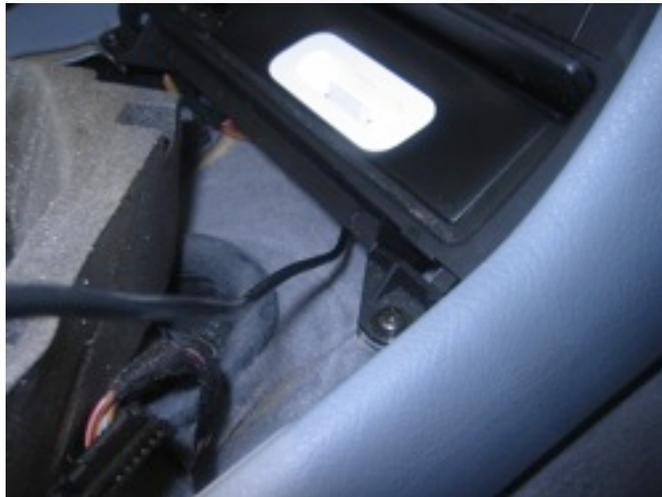
The ashtray carrier can now be reinstalled and the wiring routed to the necessary location. Reassembly of the rest of the console is the opposite of disassembly. Make sure to test all functionality before reassembling the vehicle.
