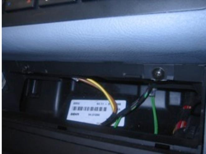
Behind this pocket are two final Philips-head screws that will need to be removed.
