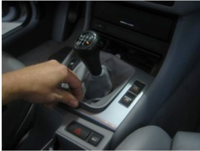
Begin by grasping the back edge of the shift boot with your fingers. The shift boot and its plastic former simply snap up out of the shifter trim as shown...
