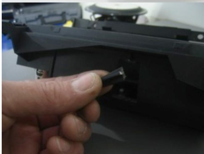
The wiring from the spec.dock will exit through this factory opening. Using your finger, push the tab outward to snap it off. This tab performs no locking or cosmetic function, so the factory ashtray can still be reinstalled at a later date.
