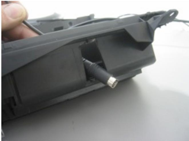
Pass the wiring from the spec.dock through this opening, feeding the cable through until the spec.dock is ready to be pressed into place.
