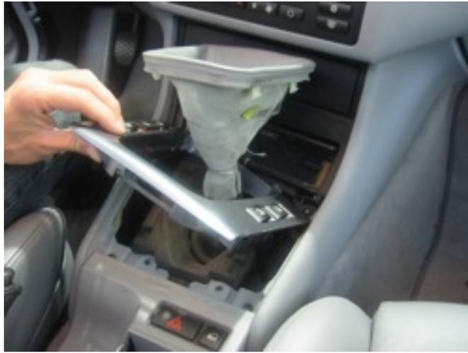
Once these screws are removed, lift up on the back edge of the shifter trim and slide it toward the back of the vehicle slightly. This will allow you to flip the piece up and unplug the wiring connectors.
