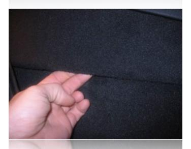
Slide your fingers in between the vehicle's carpeting and the carpeted trim on the driver's side of the center console.
