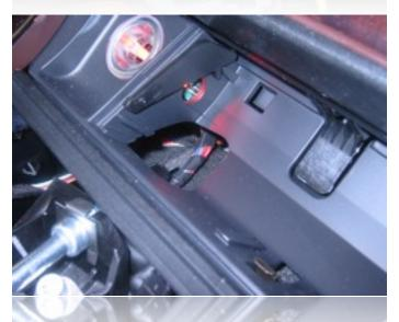
In the bottom left corner of the ashtray carrier is a factory-supplied hole that the spec.dock's wiring will pass through. Using a high-quality degreaser such as denatured alcohol, clean the ashtray carrier out completely to promote good adhesion of the spec.dock's mounting tape.
