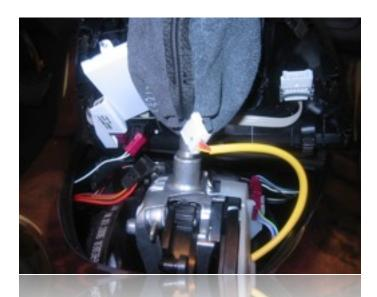
With all the connectors unplugged, you will be able to lift the shift boot and shifter trim up out of the way for access to the wire routing locations.
