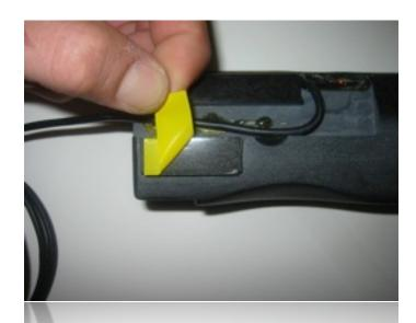
Remove the backing from the strip of tape on the bottom of the spec.dock.
