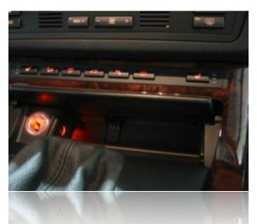
Begin by removing the factory ashtray insert by pressing back (toward the front of the vehicle) on the ashtray door. The insert will lift up slightly, allowing it to be removed.
