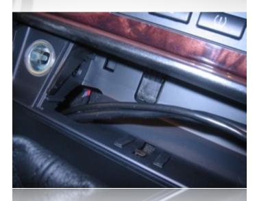
Route the spec.dock's wiring through this hole and pull it through the shift trim opening,
