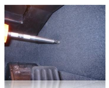
Remove the single Philips-head screw from the side of the center console toward the front of the vehicle (above the gas pedal)
