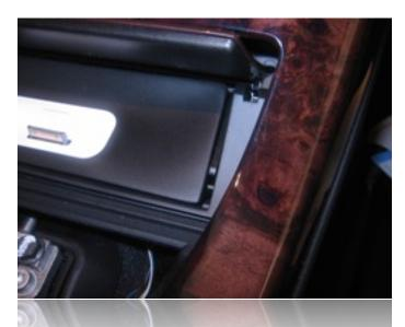
Lower the spec.dock into place while gently pulling the excess cabling from the dock through the shifter opening. Press down firmly on the spec.dock to promote good surface contact for the tape.
