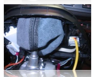
On the underside of the shifter trim are three connectors that will need to be unplugged. Disconnect these, making sure to not turn on the vehicle's ignition for the rest of the process (while these are disconnected).
