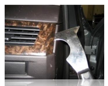
Begin by using a panel tool to pry the dash trim up on the right hand side. If the vehicle has woodgrain trim, be especially careful to pry gently, as the clearcoat on the trim will chip easily. Only move the trim out far enough to enable using your fingers to unsnap the rest of the piece.
