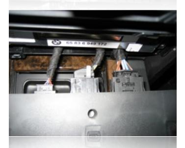
...As well as three connectors at the lower switch panel that need to be disconnected. Once these are all unplugged, the radio bezel can be removed at set aside. Make sure to not turn on the vehicle ignition once these connectors are unplugged. Do not turn the vehicle key on until all connectors have been reattached.
