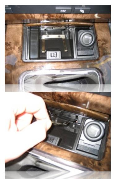
Now, turn your attention to the ashtray well. There is a small brass spring that must be removed for the spec.dock to seat properly. This can be removed by hand as shown.
