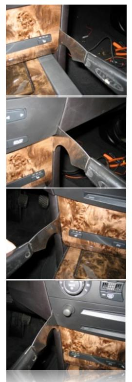
Next, carefully insert a panel tool between the radio trim bezel and the surrounding dash area in the locations indicated above and gently pry to release the clips that hold this piece in place. Again, be careful if the trim is woodgrain not to chip the clearcoat. The entire piece, including the climate controls and lower switch panel will come off together.
