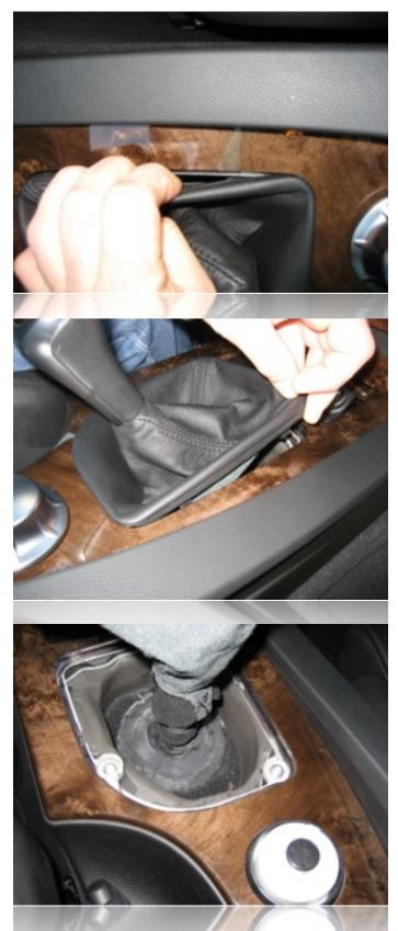
Unclip the shift boot as shown, which will expose two Torx T-20 screws, which need to be removed.
