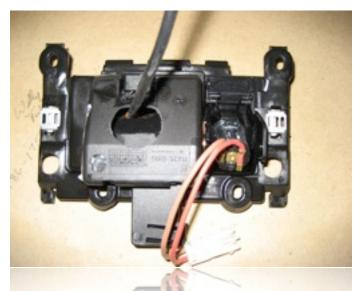
You will want to reinstall the ashtray carrier and shifter trim before permanently seating the spec.dock into position, as the retracting mechanism on the backside of the ashtray door can easily damage the spec.dock's face if the trim is not reinstalled before seating spec.dock.
