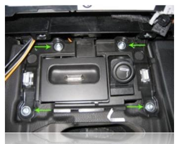
Removing the shifter trim reveals four Torx T-20 screws around the ashtray carrier that need to be removed.
