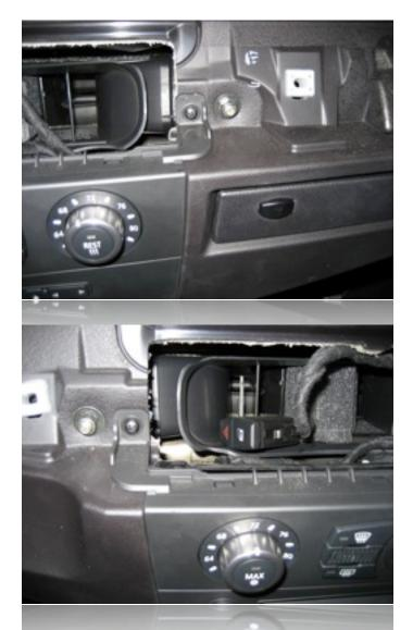
Once the trimpiece is removed and set aside, you will see two Philips-head screws that must be removed to release the radio trim bezel.
