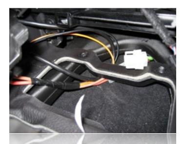
When reinstalling the ashtray carrier into the vehicle, be sure to route the spec.dock's wiring as shown to ensure a proper fit. This is how the factory cigarette lighter wiring was run when before the carrier was removed in earlier steps.
