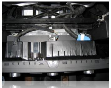
Once unsnapped from the dash, you will see a row of three connectors at the climate control module that need to be disconnected
