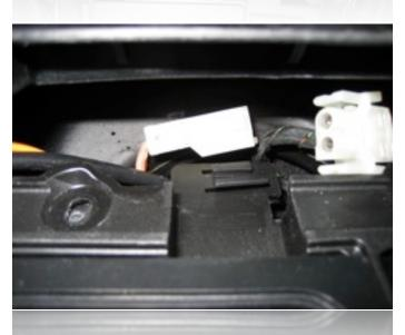
The cigarette lighter power plug must be disconnected and unclipped from the ashtray carrier so that it can be fully removed. The female side of the plug slides toward the driver's side of the vehicle to release.
