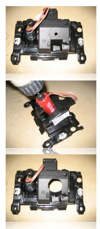
Place the ashtray carrier upside-down on a well-lit work surface and cut a 3/4" hole in the location indicated with a hole saw. This will allow the spec.dock's wiring to pass through the ashtray carrier.
