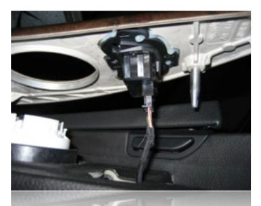
There is one connector plugged into the back of the menu and voice control buttons that will need to be disconnected. The shifter trim can now be removed and set aside.
