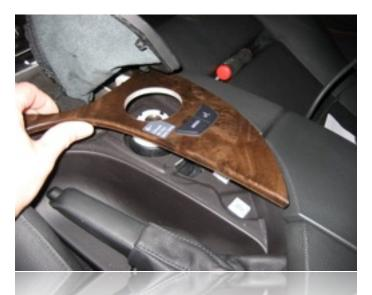
Next, use your fingers and a panel tool (if necessary) to unclip the shifter trim from the console. The front of this piece is held in place by the two screws that were removed, while the back is held in place by two clips. Be careful not to lift from the center. Instead, work your way around the back of the piece to gently release the clips. **This part is very thin and can be cracked if caution is not used in its removal.**
