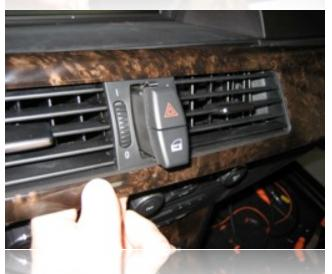
Reach in behind the trimpiece before fully removing it and pop out the hazard light/ door lock switch so that it can be easily unplugged.
