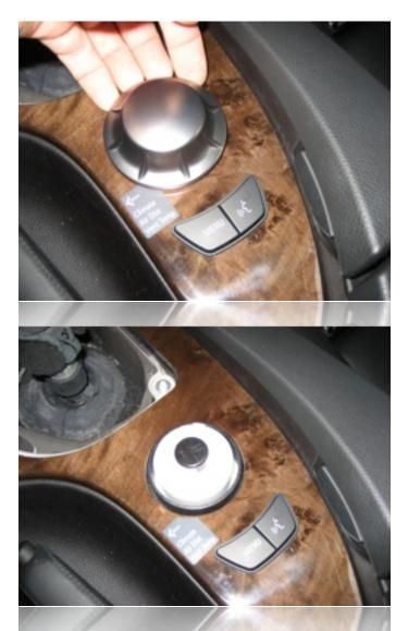
Now remove the iDrive control knob by simply sliding your fingers under its edge and lifting up slightly. The knob will unsnap easily.
