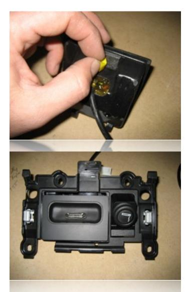
Remove the backing from the supplied double-sided tape and lower the dock into position as shown (remember, this will be done in the car - the above photo is for illustration only). Before seating the dock, be sure to clean the mounting location in the ashtray carrier thoroughly with a high-quality degreaser such as denatured alcohol to promote proper adhesion.
