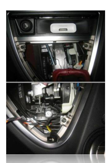
Underneath the shifter trim bezel are three more Philips head screws to remove.
