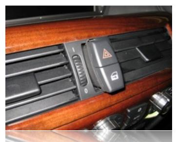
Begin by **gently** prying the hazard and door lock button assembly out of the dash trim. This is quite possibly the most delicate and difficult part of the installation process. It is not recommended to use any metallic tool. There are specially designed plastic panel tools that are quite effective at removing this switch, which most installation professionals should have at their disposal. Cosmetic damage to the trim and switches can occur if extreme caution is not used.
