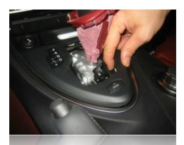
After unsnapping and lifting the shift boot out of the way, use only your fingers again and unsnap the trim bezel around the shifter as shown.
