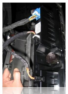
Behind the climate controls in the radio trim piece you just removed, you will see three plugs that must be disconnected. Unplug these and set the radio trim piece aside.
