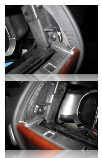
After removing the air vents, you will see two Phillips-head screws to be removed.
