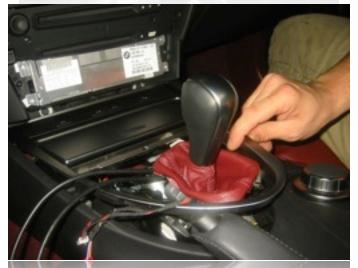
Once these screws are removed, you can begin to lift the final trim piece around the shifter out of the console. This piece includes the ashtray location where the spec.dock will be mounted.
