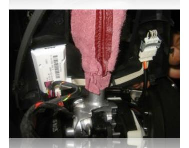
On the backside of the trim bezel around the shifter are three plugs to be disconnected. Unplug these to completely remove the shifter trim and set aside.
