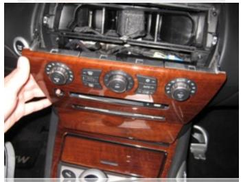
Once these have been removed, use only your hands to unsnap the trim around the radio as shown. Be careful to unsnap the clips all the way around before attempting to fully remove this piece.
