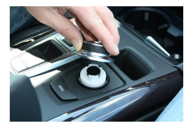
Begin by removing the iDrive knob as shown. It simply unsnaps with a little pressure. You will not need to use any tools to complete this step.
