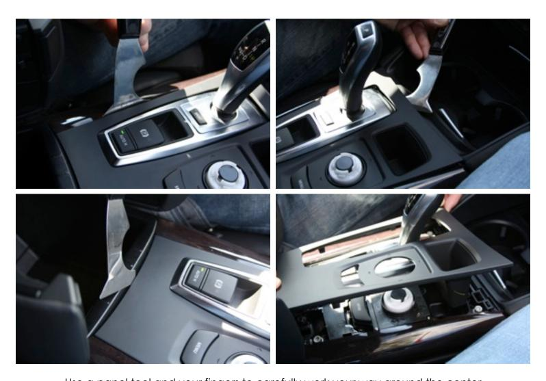
Use a panel tool and your fingers to carefully work your way around the center console trim to unsnap it from the console. The clips are fairly strong, and the woodgrain surrounding this piece is delicate, so be very careful not to chip or scratch it as you work the clips loose.
