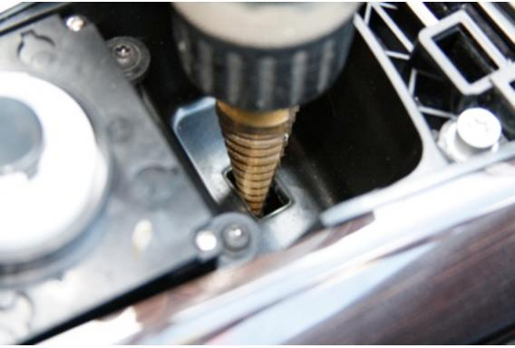
Next, use a UniBit to create a hole for the spec.dock cable to pass through in the base of the pocket, and to enlarge the original clip receptacle in the console base as shown. Be careful to check beneath the clip receptacle for wiring before drilling, and only drill as small a hole as needed.
