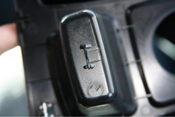
Use a pair of crimpers or other cutting tool to remove the clip on the base of the storage pocket where the spec.dock installs. This clip is redundant, and impedes the routing of the spec.dock cable through the console.
