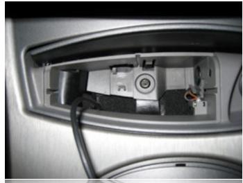
Next, remove the single Torx T-20 screw located in the ashtray carrier's base.
