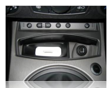
After dropping the spec.dock completely into position, press down firmly on the outer edges of the spec.dock to ensure proper adhesion of the double-sided tape. Verify all interface functions and enjoy!
