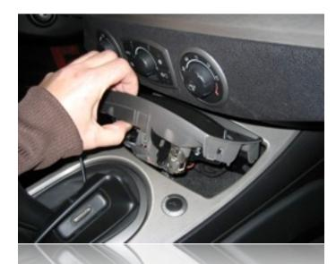
As the ashtray carrier unsnaps. Lift the front edge up and toward you to clear the dash overhang. This piece will come completely free from the console and can be set aside with the electrical connectors still plugged into the switch panel.
