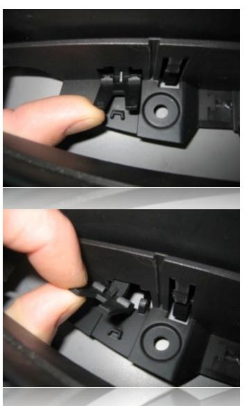
Begin by removing the ashtray lift tab from the ashtray carrier by snapping it out with your finger as shown.
