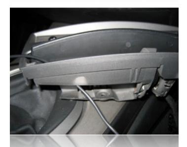
Route the spec.dock's wiring through the ashtray carrier as shown and run to the appropriate location for connection to your vehicle's audio system (see interface instructions). At this point, you can begin to reinstall the ashtray carrier into the console. **Do not mount the spec.dock until this piece is reinstalled in the console.**
