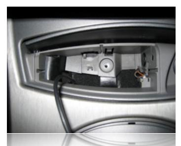
The completed wiring portion should look like this. Note that the Torx screw is not reinstalled. It will be permanently left out, as the clips hold the ashtray carrier firmly in place, and reinstalling the screw would require removing the spec.dock each time vehicle service in this area needs to be performed
