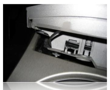
As you lower the ashtray carrier into its final position, make sure that the spec.dock's cable is routed as shown. This will prevent it from getting pinched between the ashtray carrier and any surrounding materials. Snap the ashtray carrier back in completely before proceeding to the next step.
