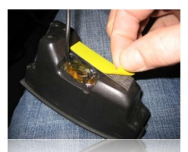
After cleaning the inside of the ashtray carrier with a high-quality degreaser such as denatured alcohol, remove the backing from the supplied double-sided tape that is attached to the spec.dock's base and lower the spec.dock into position while tucking any additional cabling into the openings between the ashtray carrier and the floor of the vehicle.
