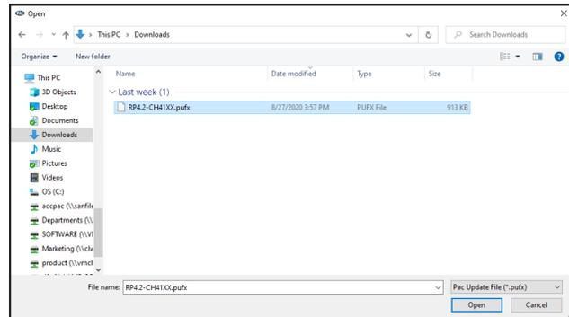
Now, select “Select File”. Finally, browse to the place where you saved the file, and select it. This will begin the updating process. Once finished, disconnect the interface from the PC. Repeat for every module: CH4A, PL1, HD1, and test operation.
