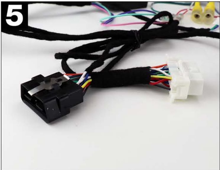
5 OBD Split Connector. Remove the vehilces OBD plug from its location and plug the white connector from the CAN104-LR01 in to this OBD socket. Position the black connector on the CAN104-LR01 in the location of the original OEM connector.
