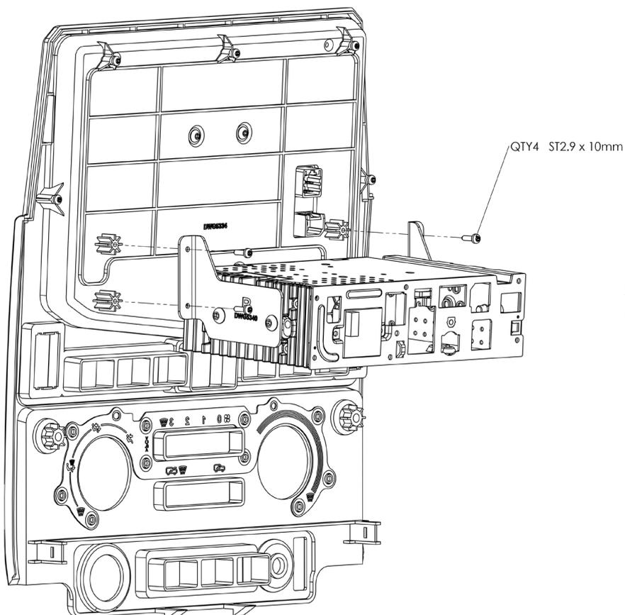
Securely affix the assembled Heigh10 chassis to the aftermarket panel using the provided ST2.9x10mm screws.
