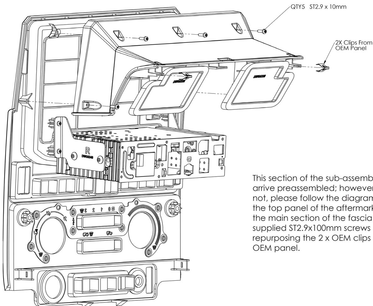
This section of the sub-assembly should arrive preassembled; however, if it does not, please follow the diagram to attach the top panel of the aftermarket fascia to the main section of the fascia using the supplied ST2.9x100mm screws and repurposing the 2 x OEM clips from the OEM panel.
