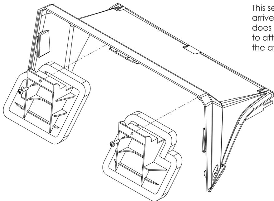
This section of the sub-assembly should arrive preassembled; however, if it does not, please follow the diagram to attach the vents to the top panel of the aftermarket fascia.
