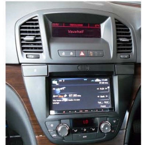
Complete installation of the aftermarket head unit
