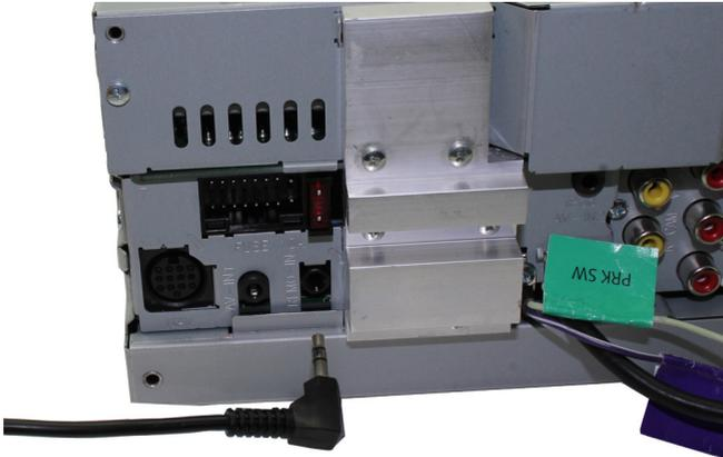
4. Connect the 14 way molex connector, the car display connector (from the vehicle) and the chime retention box to the interface.
