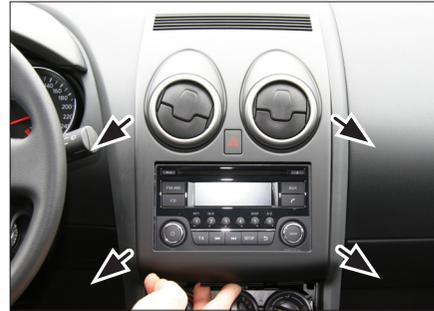
4. Unclip and remove OEM panel
