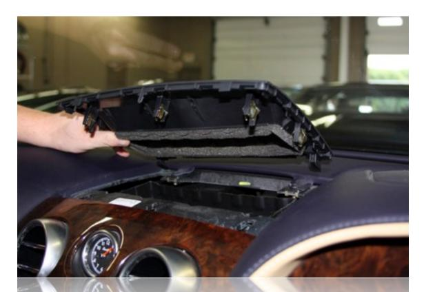
This panel simply clips in, and should be easily removed. Set aside.
