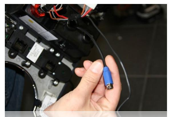
Route the connector from the spec.dock through the hole you just enlarged.
