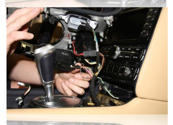
...And a few more near the shifter opening. Remove the console trim from the vehicle.
