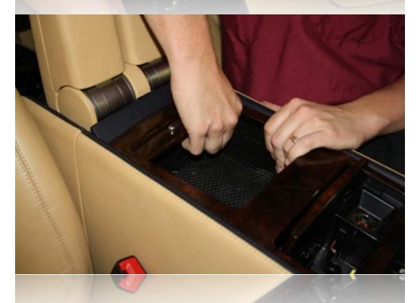
Lift the armrest, and begin unsnapping the center console trim at the storage compartment using only your hands. This piece should also unsnap easily.
