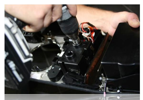
Flip the console trim over and enlarge the hole shown above in the center of the ashtray housing using a step-drill bit.
