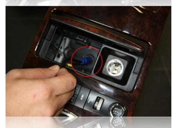
The hole should only be enlarged enough to pass the spec.dock connector through.
