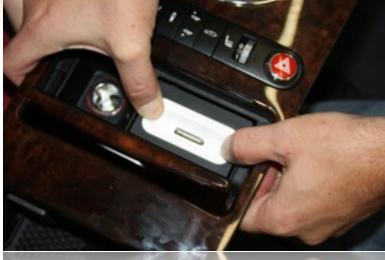
After cleaning the inside of the ashtray housing with a high-quality degreaser such as denatured alcohol, remove the backing from the pre-installed double-sided tape and lower the spec.dock into position, pressing firmly on the face of the spec.dock to ensure proper adhesion.
