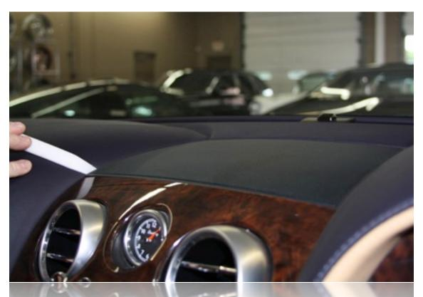
Begin by using a plastic panel tool to pry up on the front edge of the metal vent/grille at the top of the center stack. Be careful not to damage the leather dash pad.
